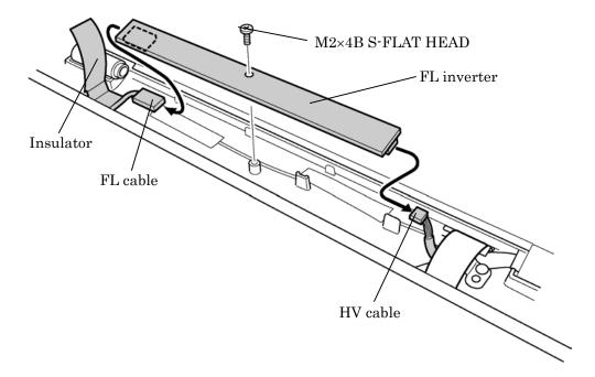
Figure 4-39 Removing the FL inverter
